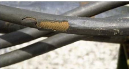
Figure 5.5.c. Hydraulic hoses may be reinforced, but damage to the outer covering—plus pin holes from high pressure—can cause serious injury (e.g. amputation) and machinery down time.
