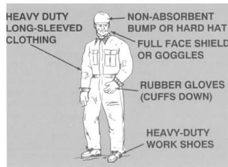
Figure 3.12.a. Personal protective equipment for working with anhydrous ammonia lowers the risk of being exposed to the burning effects of the \text{NH}_3 on the skin, the eyes, and the lungs. Farm and Ranch Safety Management, John Deere Publishing, 1994. Illustrations reproduced by permission. All rights reserved.
