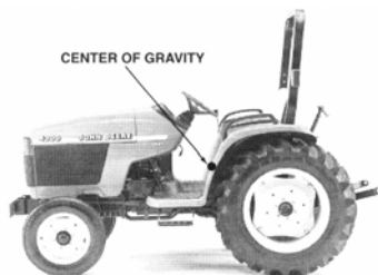
Figure 4.12.a. Expected position of a tractor's center of gravity. Safety Management for Landscapers, Grounds-Care Businesses, and Golf Courses, John Deere Publishing, 2001. Illustrations reproduced by permission. All rights reserved.
