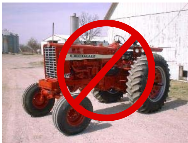
Figure 4.2.d. Older tractors are often assigned to younger drivers to do less heavy chores. Raking hay, pulling wagons, and hauling feed to livestock does not require the most powerful tractor. Older tractors may have safety deficiencies due to age and missing safety features. This tractor does not have a ROPS or seat belt.
