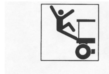
Figure 2.8.f. This safety sign warns of a potential fall hazard. Always use handholds. Falls account for a large number of agricultural injuries and fatalities each year.
