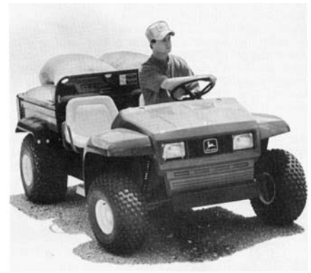
Figure 6.2.c. A utility vehicle is versatile. It can do the smaller jobs that a pick-up truck may be unsuited to do. Remember that the utility vehicle has limitations. Overloading, shifting loads, and sharp braking can cause turnovers.
