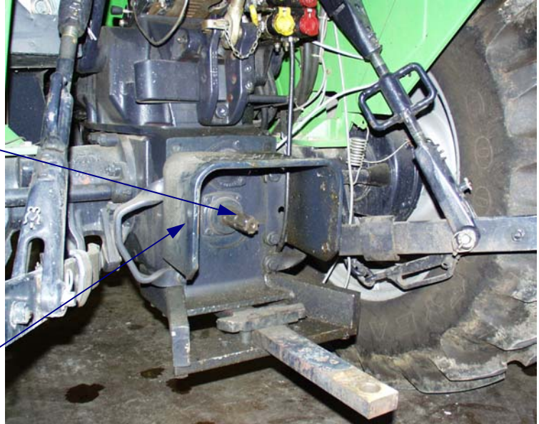
Figure 5.4.1.b. The major components of a PTO system found on the tractor.
