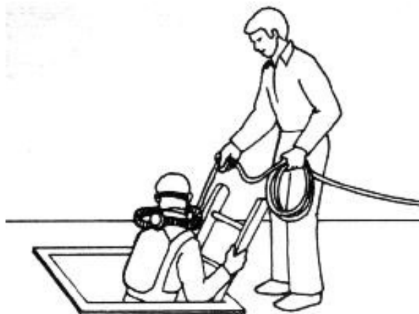
Figure 3.11.d. The only safe way to enter a manure pit is by using a self-contained breathing apparatus (SCBA). Only trained persons should use the SCBA. A lifeline is also a part of safe entry.
