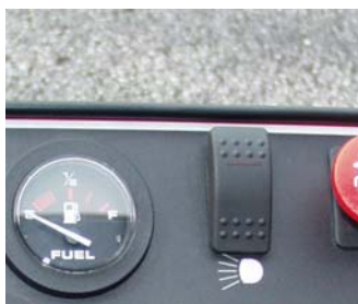
Figure 4.5.4.c. The light control switch is a black rocker switch.
