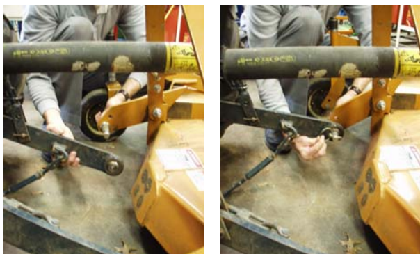
Figure 5.3.c. On both the left and right sides of the implement, insert the draft arm attachment pin of the tractor into the pin holes of the implement's lower hitch assembly. Secure the hitch with the proper size hitch pins and security clip.
