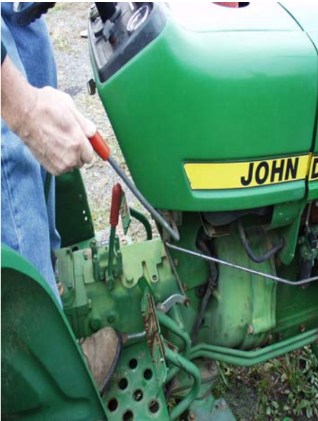
Figure 4.5.1.b. Diesel engines are often stopped by shutting off the fuel flow from the fuel pump.
