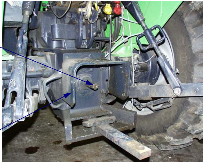
Figure 3.1.b. A PTO stub and a master shield on a tractor. A PTO is a wrap point hazard that causes countless injuries and deaths each year.
