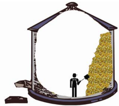
Figure 3.10.f. Damp, moldy grain can stick to the side of the grain bin. It can collapse on the worker who tries to dislodge it.
