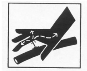
Figure 2.8.h. A potential high pressure hydraulic hose leak is a hazard which could force oil beneath your skin. Check hydraulic leaks with a mirror or piece of metal instead of your hand or fingers.
