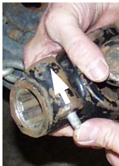
Figure 5.3.e. A firm grip will be needed to press in on the detent lock of the PTO shaft. This lock engages the groove in the stub shaft to secure the PTO driveline shaft to the stub shaft. Other forms of locking the PTO shaft will be found in Task Sheet 5.4.
