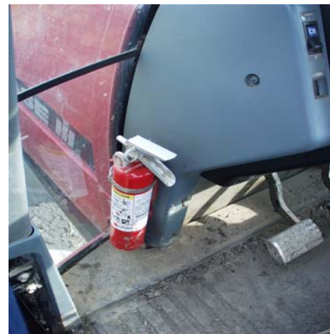
Figure 3.7.1.e. All tractors should have a dry, chemical- type fire extinguisher on board. Today's high-priced tractors and equipment should be fire control ready. What class(es) of fire will the dry chemical extinguisher control?
