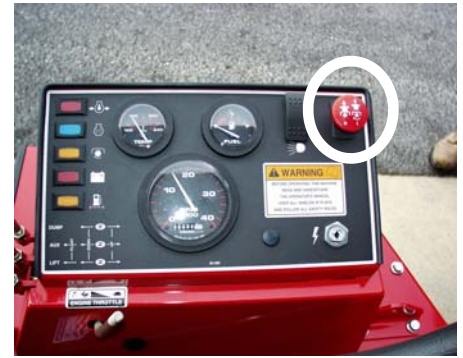
Figure 4.5.5.h. Engine stop control —A key switch must be rotated counterclockwise to stop the engine. A mechanical pull-push control must be within 6 inches of the key switch and pulled to stop the engine. Engine stop and ground speed controls that are combined into a single lever must move in the same direction to first slow ground speed and then stop the engine.
