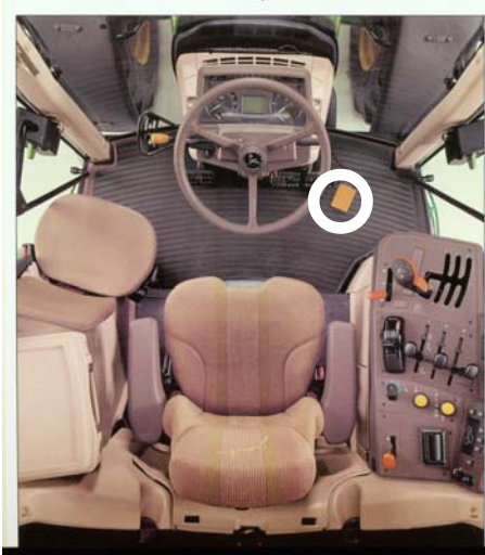
Figure 4.5.2.b. The foot throttle on the tractor is orange in color. Orange is the color code for ground motion controls.
