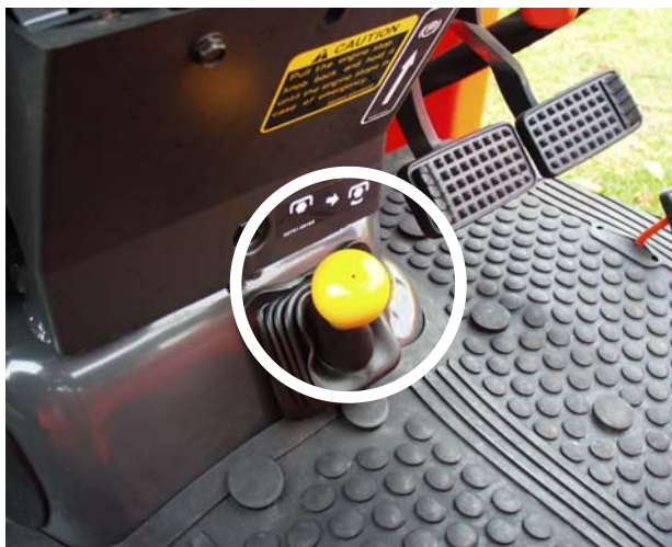
Figure 4.5.3.a. Yellow color-coded controls engage accessories. This is often done through the PTO.
