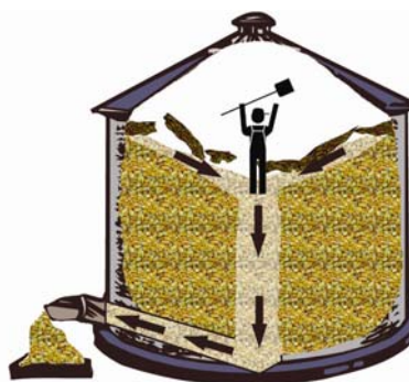
Figure 3.10.e. As the grain bridge gives way, the worker is pulled into the pocket and is engulfed. The grain auger may have been left running and the flowing grain pulls the victim under the grain.
