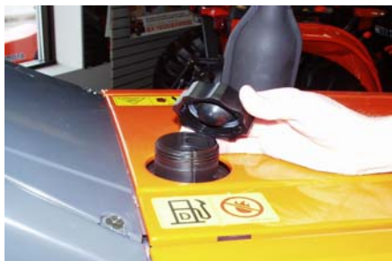
Fig. 4.6.1.b. Check the fuel level.
