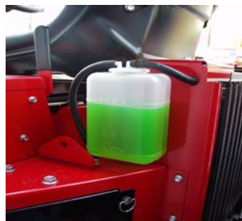
Fig. 4.6.1.d. Check the coolant level with the engine cold.
