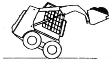
Figure 6.1.c. Skid steer loaders can tip forward if overloaded. This is an important reason to wear the seat belt, as well as understand the skid loader's load limitations.
