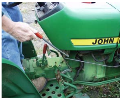
Figure 4.7.f. Set the throttle to 1/3 of its working range.
