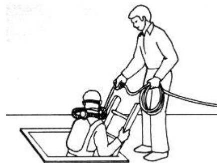
Figure 3.8.d. Confined space entry into oxygen-deficient areas requires SCBA. Training is necessary to use this equipment.
