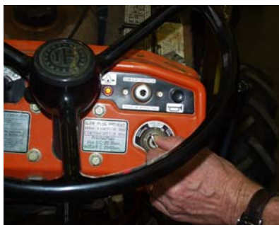
Figure 4.7.e. Be sure fuel pump shut-off knob is in the "on" position. If the conditions are cold, turn the ignition key to the glow plug setting and hold until the indicator shows that the combustion chamber is hot enough to ignite the diesel fuel droplets. If you don't know how to do this, ask someone to show you.
