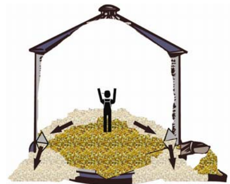
Figure 3.10.g. It takes much force to remove a grain bin entrapment victim. Rather than removing the victim, it is easier to remove the grain. Special tools and skills are needed to cut through grain bins and remove the grain.
