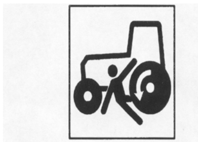
Figure 2.8.i. This safety sign warns of the potential to be run over by a tractor. Use the seat belt while operating the tractor equipped with a ROPS. Do not stand to drive. Passengers should not be allowed to ride the tractor. Extra riders are at a great risk for injury or death.
