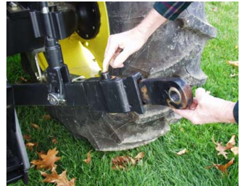
Figure 5.3.h. If the 3-point hitch is equipped with an extension to the lower draft arm, release the lock and pull or extend the draft arm extension to the rear before nearing the implement to be attached.
