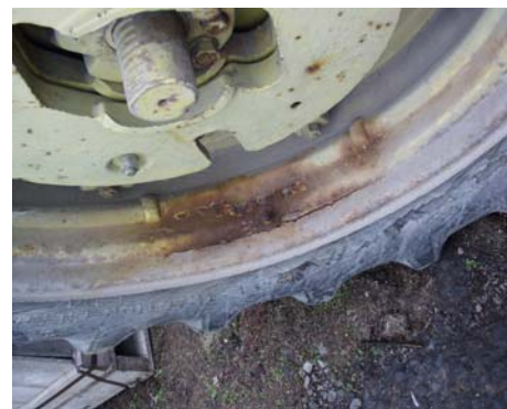
Fig. 4.6.5.d. A leaking valve stem released calcium solution which rusted the rim. A major expense will be incurred, as well as a severe safety hazard in using this tractor.
