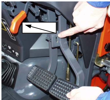
Figure 4.5.2.c. Brakes are locked together and the orange lever is for setting the brakes on this tractor.
