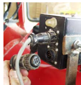
Figure 5.6.d. Align the pins of the electrical connection before attaching. Do not force the connector if the pins are not aligned. Threaded connectors do not pull loose; unscrew them first.
