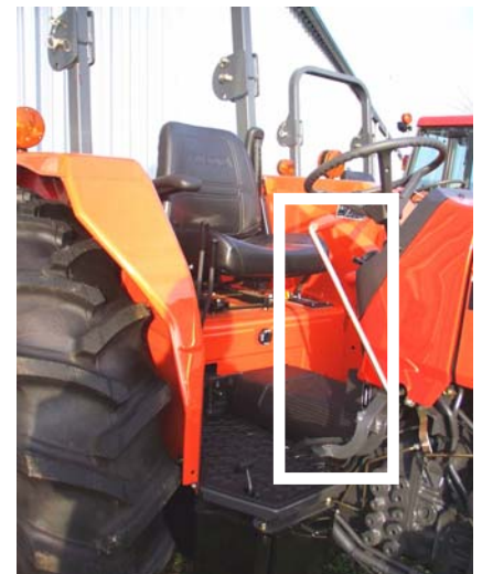
Figure 4.5.5.e. Engine speed control— The control is located on the right side. If the hand-operated control is located next to the tractor seat, the direction of motion must be forward or upward to increase engine speed and rearward or downward to slow engine speed.
