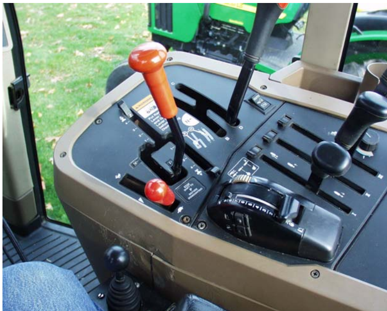
Figure 4.10.b. Be sure to study the gear shift pattern on the tractor you are operating. Use a lower gear to start moving. Use a higher gear for operation. Higher gear use with heavy loads may stall the engine or can cause rearward overturns. If the shift pattern is hard to locate, ask someone who is familiar with the tractor to show you the shift pattern.
