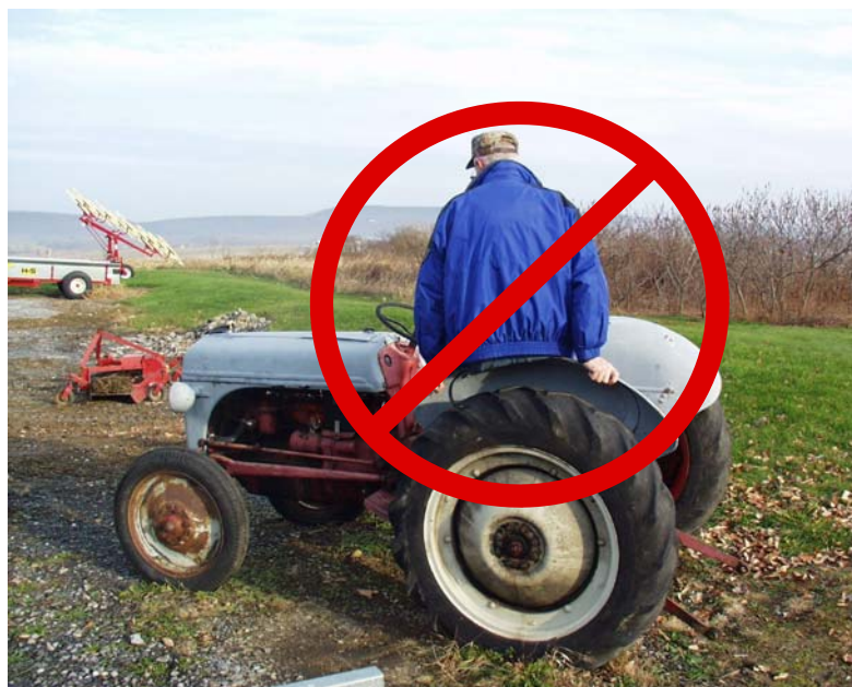
Figure 4.2.b. Tractor runovers have claimed many lives. Extra riders can slip from the tractor and be crushed before the operator can stop. Say no to your friends who want to hitch a ride.
