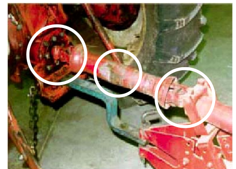
Figure 5.4.1.d. A bent shaft guard offers no protection from a spinning PTO shaft. Also notice the missing master shield and the inadequate guarding of the universal joint near the PTO pedestal.
