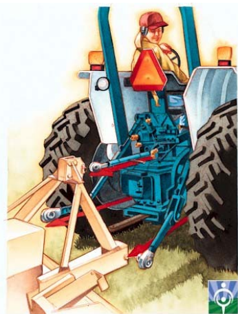
Figure 5.3.a. Back slowly to the implement to be attached. Using the hydraulic controls, raise or lower the draft arms to nearly match the implement's lower hitch pins.
