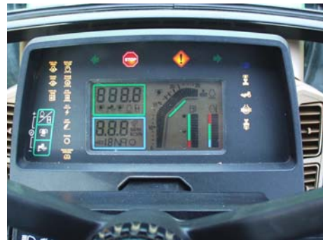
Figure 4.4.a. The modern tractor instrument panel may appear as complex as the cockpit controls of a jet airliner. The operator must know what each instrument or gauge is telling him/her about operating conditions.
