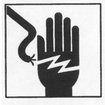
Figure 3.6.a. Contact with an electrical current can kill a person. The heart muscles will lock up if the electrical current passes through the heart when all the heart valves are closed (rest phase).
