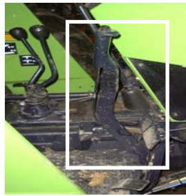
Figure 4.5.5.b. Brake control— Foot brake pedals must be located on the right side. Push the brake forward and/or downward to engage. If a hand brake is provided, it can be on either side and must be pulled to be set. Brake locks may be lifted to be set.
