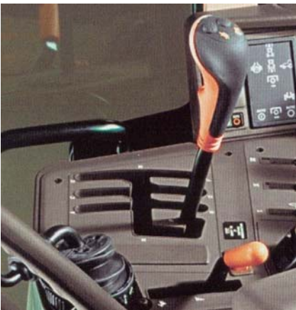
Figure 4.5.5.f. Ground speed control —A hand-operated forward-reverse (non-variable speed) directional control must be moved forward for forward travel and rearward for reverse. A hand-operated variable speed control must be moved forward and/or upward to increase speed and rearward and/or downward to decrease speed.
