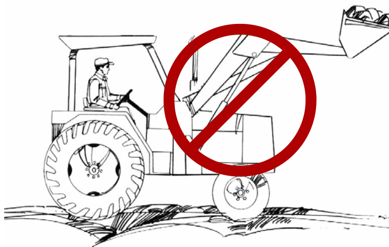
Figure 4.13.k. When operating a high-lift bucket with a load or without a load, keep the bucket as low to the ground as possible while in transport. Sideway overturns are possible if you try to travel with the bucket in the up position. Farm and Ranch Safety Management, John Deere Publishing, 1994. Illustrations reproduced by permission. All rights reserved.
