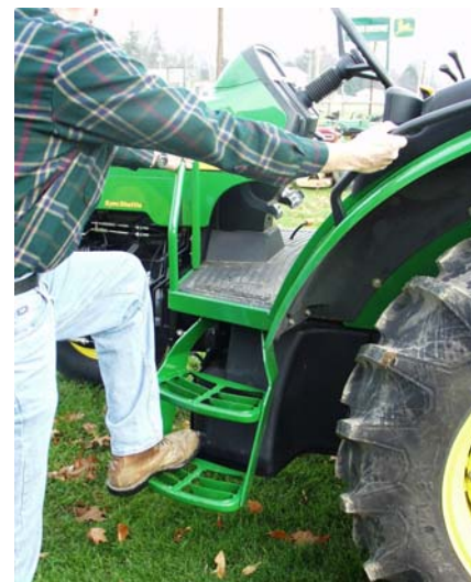
Figure 2.8.n. Use the handholds and face the steps when mounting the tractor. What hazard warning sign would you expect to see in this situation?
