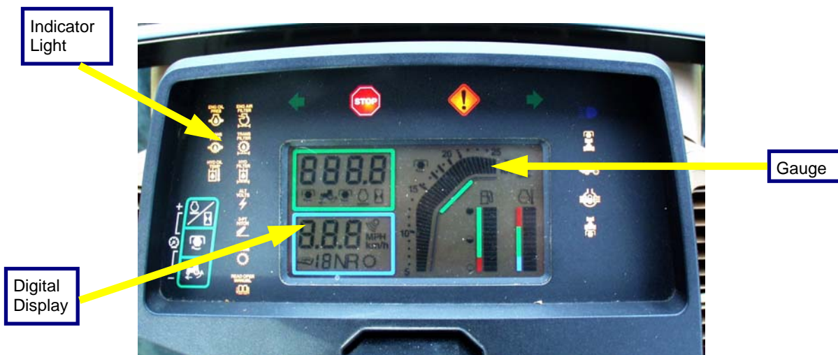
Figure 4.4.b. You may find indicator lights, standard gauges, computerized digital displays, and buzzers as instruments to show operating conditions.
