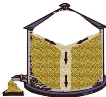
Figure 3.10.a. The normal flow of grain from a bin is off the top and down a center column of grain flowing toward the unloading auger. The unloading auger is found at the bottom center of the grain bin.
