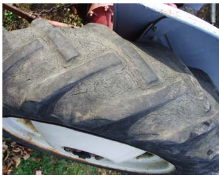
Fig. 4.6.5.b. Worn treads and dry rot make for poor traction and risk for downtime due to a blowout.
