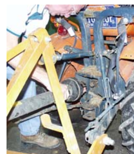
Figure 5.3.f. To attach the PTO shaft, you will be operating in a crowded space. Be sure the tractor engine is shut off and is securely parked.
