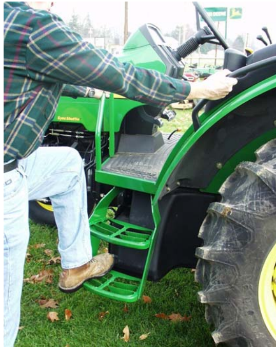
Figure 4.9.a. To prevent falls, use the handholds and footsteps provided to dismount from the tractor. Falls while dismounting account for many farm injuries each year.
