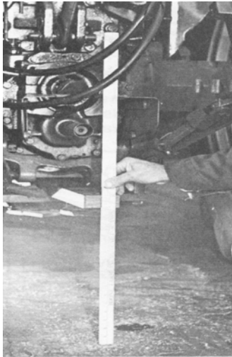
Figure 5.1.d. Tractor drawbars are designed at the correct height from the ground to keep the pull forces below the center of gravity. Only use the drawbar to tow a load. A swinging or floating drawbar permits adjustment of the center line of pull to be maintained even on a hillside.
