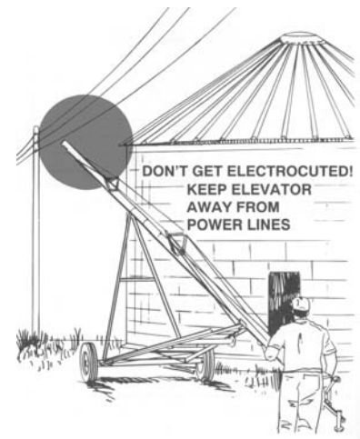
Figure 3.6.c. Lower the hay elevator or grain auger to avoid contact with overhead power lines. Farm and Ranch Safety Management, John Deere Publishing, 1994. Illustrations reproduced by permission. All rights reserved.
