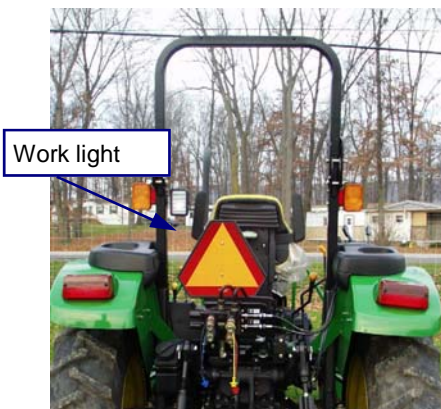
Figure 4.14.c. Be sure that a work light that points to the rear is off during road travel at night. Single white lights may not be recognized as slow-moving or as a tractor light. Also if SMV emblems are worn or obsolete, replace them with newer more reflective SMV emblems.
