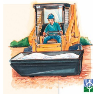
Figure 6.1.a. Skid steers are controlled by hand levers or joy sticks. Push the levers forward to travel forward; pull back to go in reverse. Let go to stop. The levers also steer the machine.
