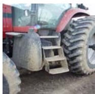
Figure 4.6.6.b. Falls account for many farm injuries. Keep the steps and platform clean of mud, manure, and tools.
