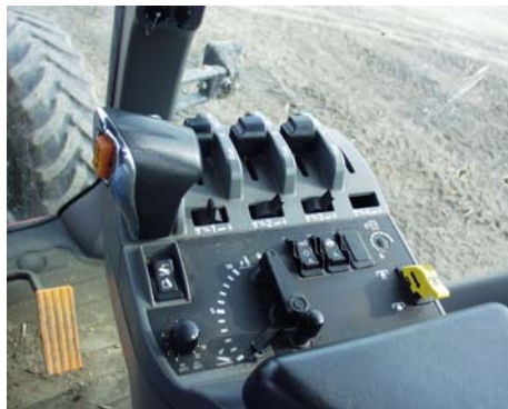
Figure 4.5.3.d. Rocker arm switches may be used. If you find a control feature with which you are unfamiliar, ask for instructions before operating costly equipment.
