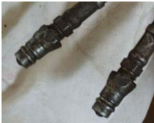
Figure 5.5.g. The male half of the coupler is part of the cylinder or hydraulic device system. Be sure to wipe dirt and grime from the hose end fitting.
