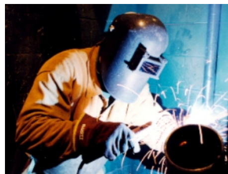
Figure 3.7.e. Welding sparks from electric arc welders and oxyacetylene gas welding equipment can create the spark that ignites nearby flammable materials or vapors.
