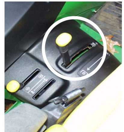
Figure 4.5.5.d. Power Take-Off (PTO) control— A hand-operated PTO control can be located on either side and will be moved upward or forward for engagement and rearward or downward for disengagement.
