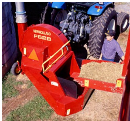
Figure 3.9.b. While filling the silo, the work is done in close quarters. Two tractors are often involved with the PTO shafts operating the self-unloading wagon and the silage blower. Extreme caution is needed to do this work safely.
