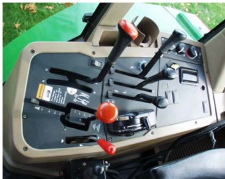
Figure 4.5.4.b. High lift controls are color-coded black.
