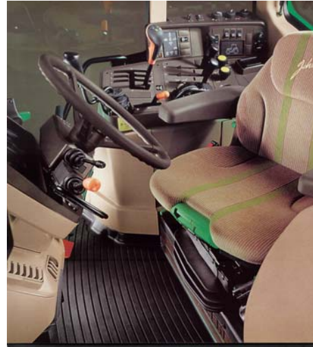
Figure 4.5.5.a. Tractor controls are placed in specific locations so that operators do not have to search for them. Older tractors may have controls placed in various locations. How the control is used may be entirely different from tractor to tractor.
