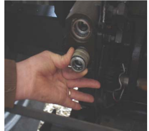
Figure 5.5.h. The lock ring of the female end of the coupling will secure the two fittings together.
