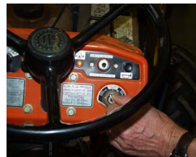
Figure 4.7.g. Turn the ignition key clockwise to the start position. Do not hold it there for extended periods of time. This can damage the starter motor or drain the battery of its charge.
