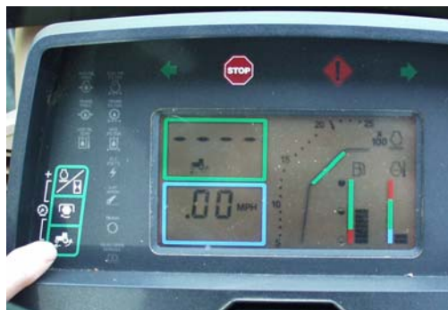
Figure 4.4.c. Check the manufacturer's RPM recommendations for various jobs to be done. Tachometers may be a gauge type or a digital display as shown above.
