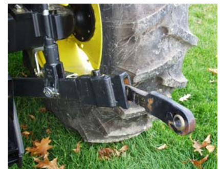
Figure 5.3.i. The telescopic extension to the draft arm is fully extended. In some cases, this must be done to align with the lower lift points of the 3-point hitch implement. Be sure the extension is pushed back into the draft arm until locked into place when you are finished attaching the implement.
