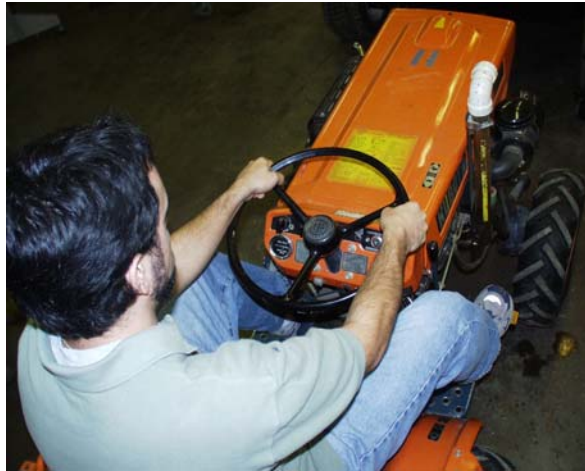
Figure 4.10.c. Use both hands to steer the tractor. If you hit a hole in the field, the wheel can be jerked from your hand.
