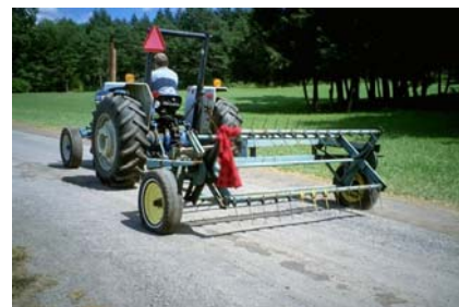
Figure 5.2.c. Implements can be wider than the tractor in transport or road position. Passing through farm gates or using public roadways can create a hazardous situation.
