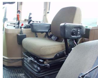
Figure 4.6.6.e. Locate seat adjustments and know how they work. You may need the Operator's Manual. Farm and Ranch Safety Management , John Deere Publishing, 1994. Illustrations reproduced by permission. All rights reserved.
