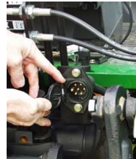
Figure 5.6.b. Electrical connectors are protected from dust, dirt, grease, and grime with dust caps. Keep these covers repaired and in place to insure that electrical connections can be made without delay.
