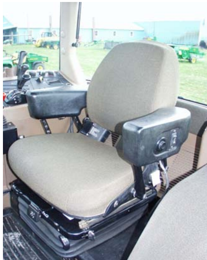
Figure 4.5.4.d. There are many seat adjustments shown here. Seat positioning and adjusting is coded with black knobs.
