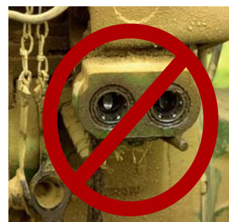
Figure 5.5.a. Missing hydraulic connection covers signify a problem with this tractor. What will happen to the hydraulic system if the dust covers are not kept in place?
