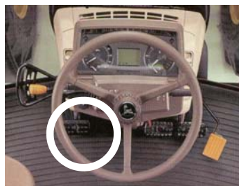
Figure 4.5.5.c. Clutch control— A foot clutch pedal must be located on the left side. The pedal is moved forward or downward for disengagement. A hand-operated clutch can be located on either side and must be moved toward the operator to be disengaged.
