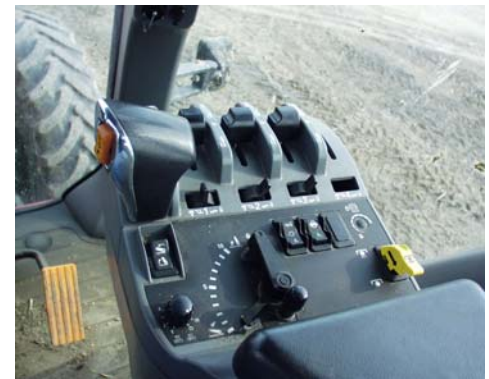
Figure 4.5.5.i. Lift controls for implements or attachments —Lift controls must be located on the right side. A hand-operated control must be moved forward, downward, or away from the operator for lowering, and backward, upward or toward the operator for lifting.
